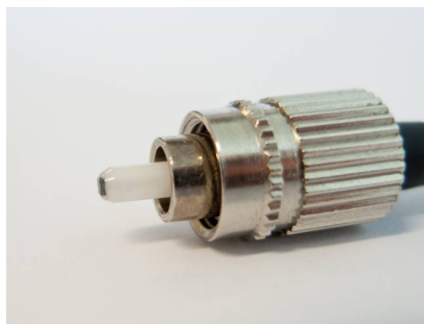
SAM chip on FC/PC connector end face
