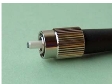
figure 1: RSAM chip on FC/PC connector end face
