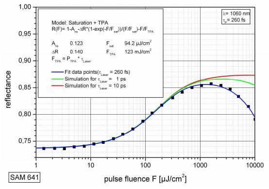
The saturation measurement has been done using a pulsed laser source with 260 fs pulse duration. Due to the high peak power density the two photon absorption (TPA) is significant in this case. The green and red curves are simulated for the same pulse fluences, but longer pulse durations of 1 ps and 10 ps respectively..
