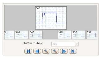
When the trace length is set to be shorter than the scope's memory, the PicoScope will automatically configure the memory as a circular buffer, recording recent waveforms for review. For example, if 1 million samples are captured, up to 500 waveforms will be stored in oscilloscope memory. Tools such as mask limit testing can then be used to scan through each waveform to identify anomalies.
