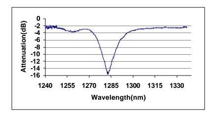
Long period grating couples light from a guide mode into forward propagating cladding modes where it is lost due to absorption and scattering. The coupling from the guided mode to cladding modes s wavelength dependent so we can obtain a spectrally selective loss.
