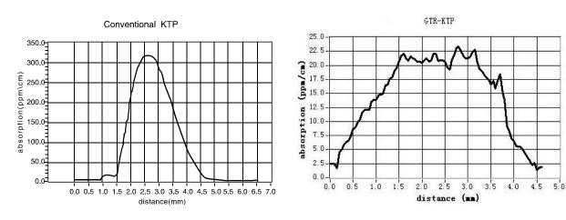
It appears that the absorption of CASTECH's GTR-KTP at 1064 nm is only 1/10 of conventional KTP.
