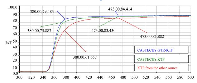
Apparently CASTECH's GTR-KTP has lower absorption than the conventional KTP in the range of 350-550 nm. We can conclude that CASTECH's GTR-KTP is expected to have a higher gray tracking resistance than the regular flux grown KTP crystals.
