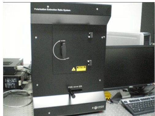
Extinction Ratio Measurement PER:>50dB ER:>250000:1
