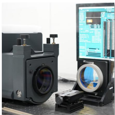
ZYGO Interferometer: parallelism & wave front Parallelism measure accuracy: 0.5 "
